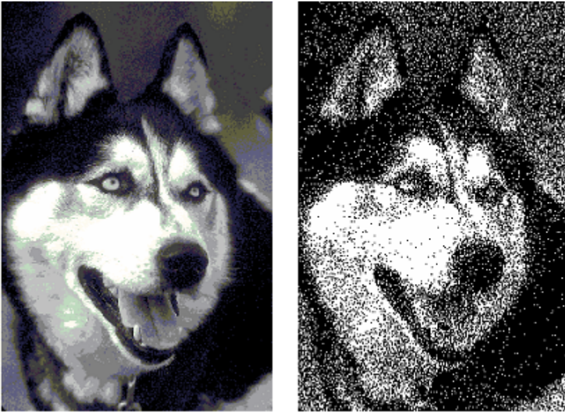
Figure 165: original picture (left) and scanner image in error diffuse mode (right)
